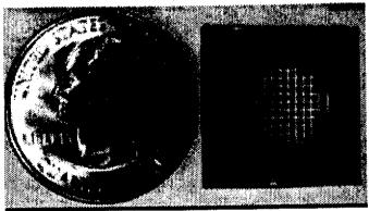
A carbon-nanotube membrane (quarter shown for scale). The nanotubes are located at the center of each square. Despite their tiny size, they can filter water more efficiently than current larger membranes. (Credit: Science)
